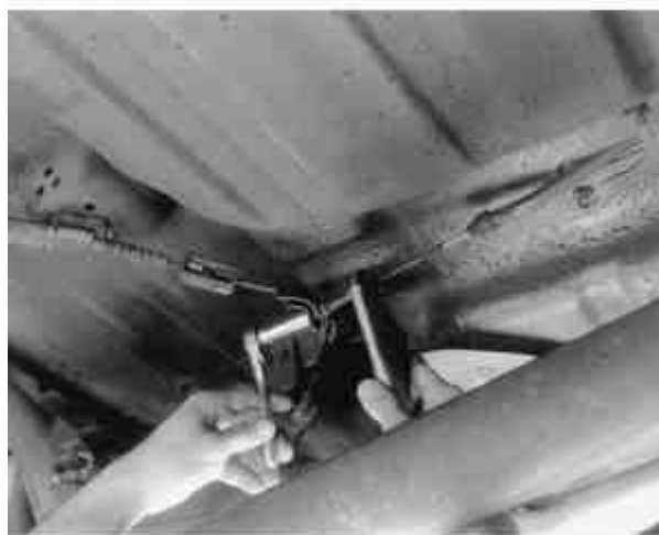
Fig. 3: View of the brake warning lamp switch — note
