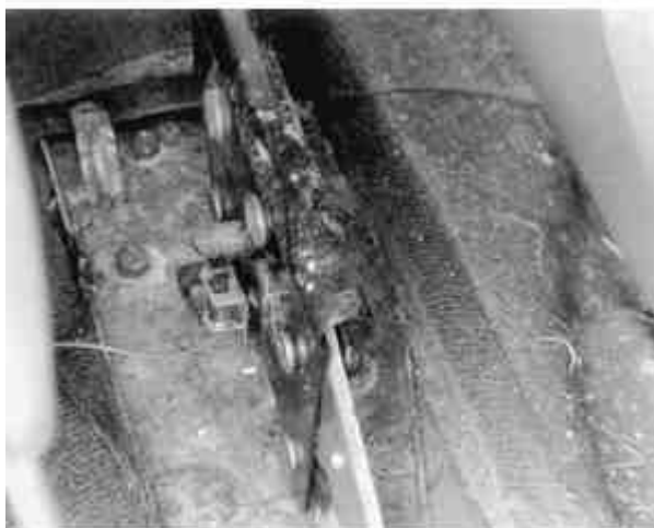
Fig. 4: If necessary, bend the brake warning lamp switch plate to adjust the lamp's activation
